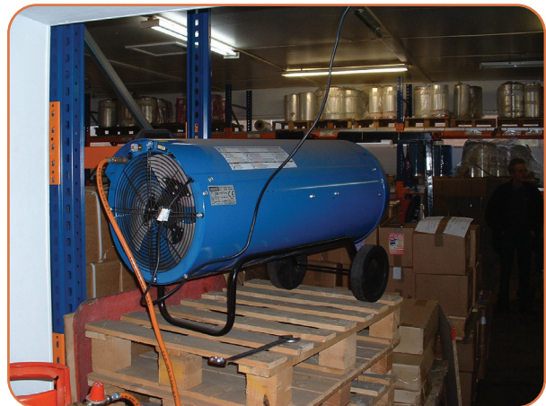
Figure 2-13: Mobile ignition source. Source: FSTC Ltd.
